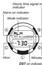
When the Daily Alarm is turned on, the alarm sounds for 20 seconds at the preset time each day. Press any button to stop the alarm after it starts to sound. When the Hourly Time Signal is turned on, the watch beeps every hour on the hour.
