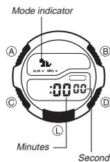
The Easy Timer Mode lets you quickly and easily set a countdown timer within the range of 1 to 60 minutes. When the end of the countdown is reached, an alarm sounds for 10 seconds, or until you press any button on the watch. When the alarm stops, the countdown start time is cleared automatically.
